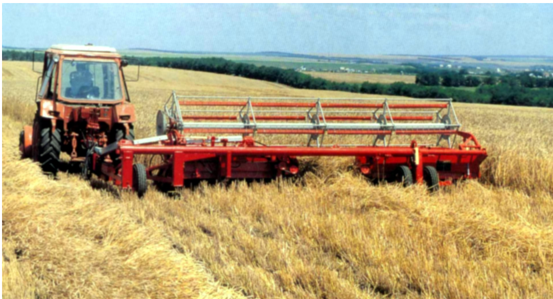
Fig. 1. Asymmetric swath reaper aggregate, prepared for experimental field investigations
