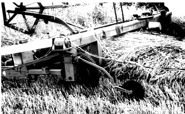
Fig. 2. Track-measuring wheel, installed on trailed swath reaper
